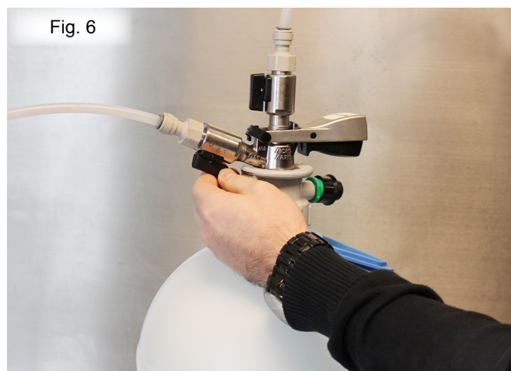
If you have shut-off valve on your dispense head, you should open it.
